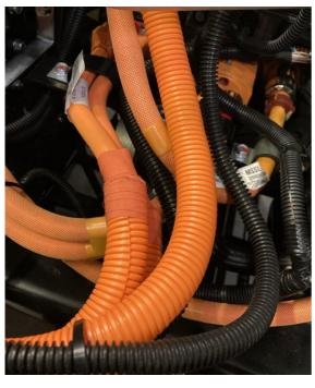
HV cable with basic insulation and protection
